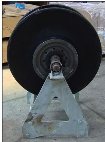
2. Rotate rotor and allow to wind down, heaviest point will be at bottom.
